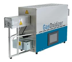
To guarantee that all sulfur compounds can be measured in the exhaust gas as  $S0_2$ , the V&F GasOxidizer is applied. With this device all sulfur compounds are oxidized to  $S0_2$  by adding a mixture of oxygen  $(0_2)$  and ozone  $(0_3)$ . For the quantitative determination of  $S0_2$  in car exhaust gases the sensitive ion molecule reaction (IMR-MS) mass spectrometry is applied.
