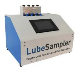
The engine lube oil can be sampled continuously via a circulation pump. Using a spindle valve a small portion of the oil can be injected into the integrated partial pressure generator. There the separation of the fuel and the oil takes place via thermal desorbtion.
